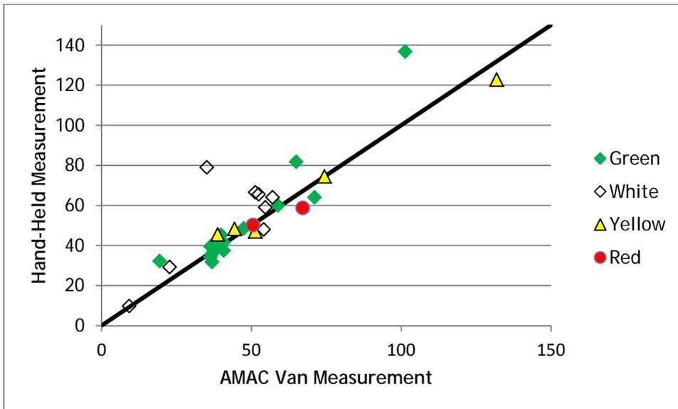
Figure 10. Close-Up of Comparison of Background Measurements ( $\text{cd/lx/m}^2$ )
