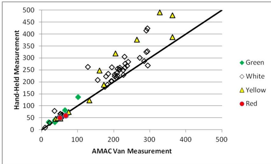
Figure 9. Comparison of Background Measurements ( $\text{cd/lx/m}^2$ )
