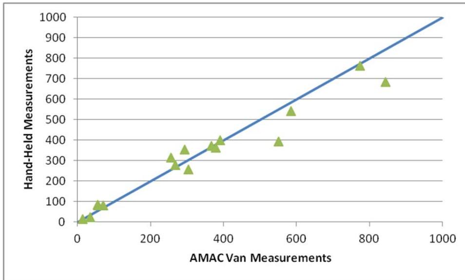
**Figure 5. Comparison of Legend Retroreflectivity Measurements (cd/lx/m<sup>2</sup>)**
