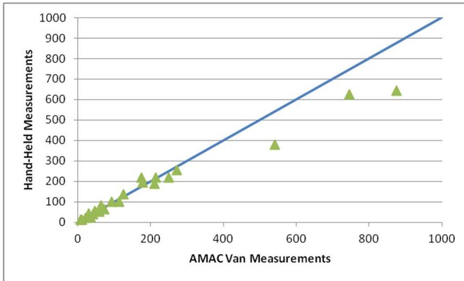
**Figure 4. Comparison of Background Retroreflectivity Measurements (cd/lx/m<sup>2</sup>)**
